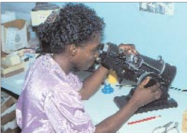
Recording the spectacle lens powers using the focimeter
